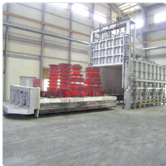
■ Heat Treatment Furnace
